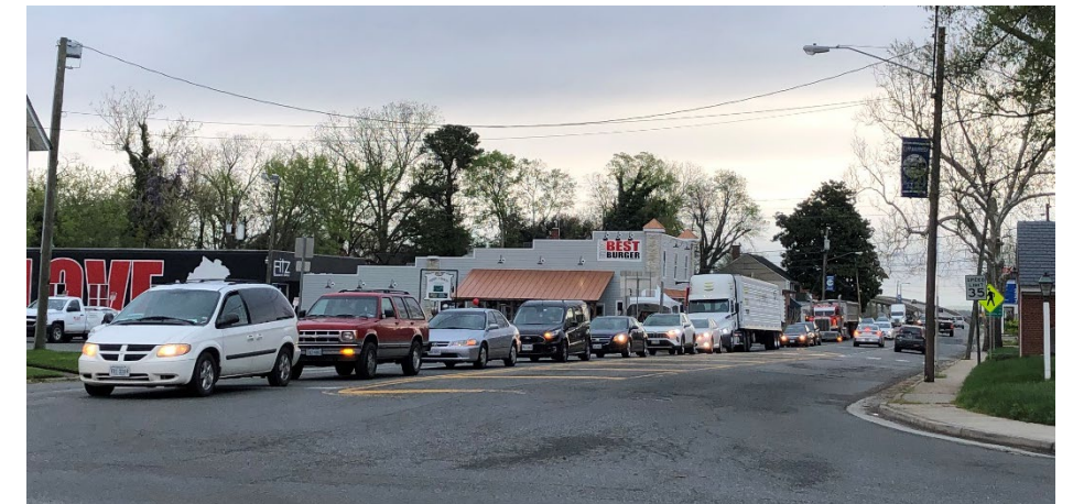
THE WESTBOUND QUEEN STREET QUEUE FROM THE TRAFFIC SIGNAL AT US 17 (CHURCH LANE) CONSISTENTLY QUEUES BACK BEYOND CROSS STREET IN THE AM PEAK HOUR.
