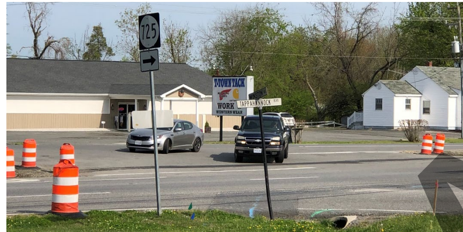
EXAMPLE OF DOUBLE-STACKING IN THE MEDIAN AT WINSTON ROAD AND IMPROPER VEHICLE POSITIONING.
