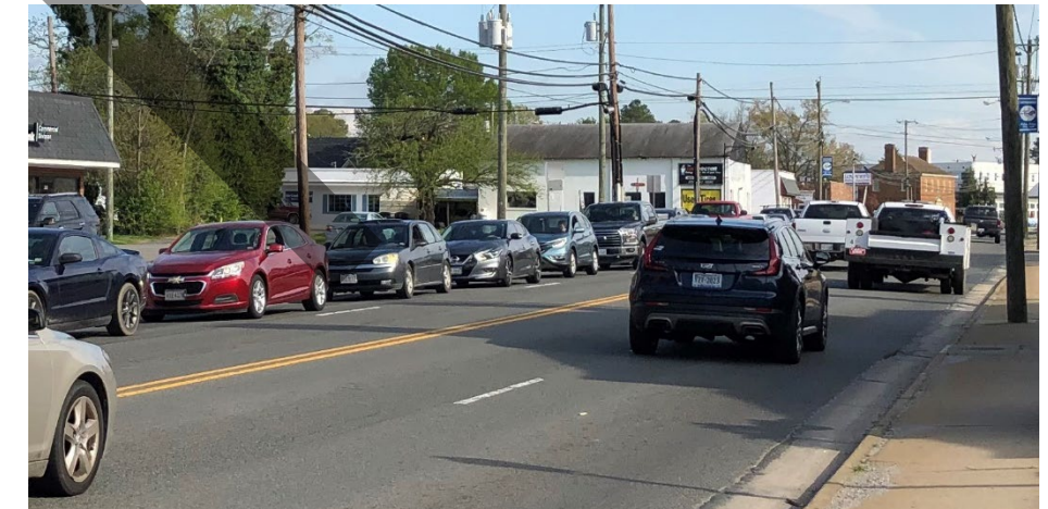
THE NORTHBOUND QUEUE ON US 17/360 FROM QUEEN STREET EXTENDS BACK TO DUKE STREET, BLOCKING THE WESTBOUND APPROACH OF DUKE STREET.
