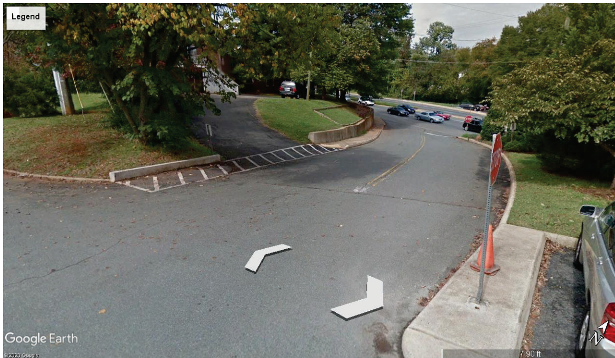
Figure 25. Entrance to Burnley-Moran off of Long St is missing a continuous sidewalk (Google Street View, 2020)
