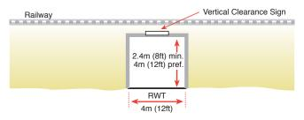
FIGURE 5.31 RWT culvert under tracks
