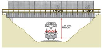
FIGURE 5.34 RWT track overcrossing (meets Amtrak required clearance height for non-electrified track)
