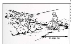
**Figure 15-11.** GOOD DESIGN: A turning area with a slope equal to or less than 5 percent in any direction enhances access on a trail with switchbacks.
