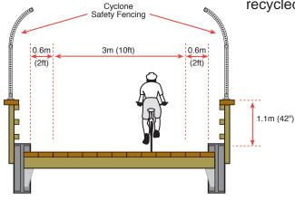
FIGURE 5.33 RWT track overcrossing Railroad Overcrossing Cross Section (Rails-With-Trails: Lessons Learned)
