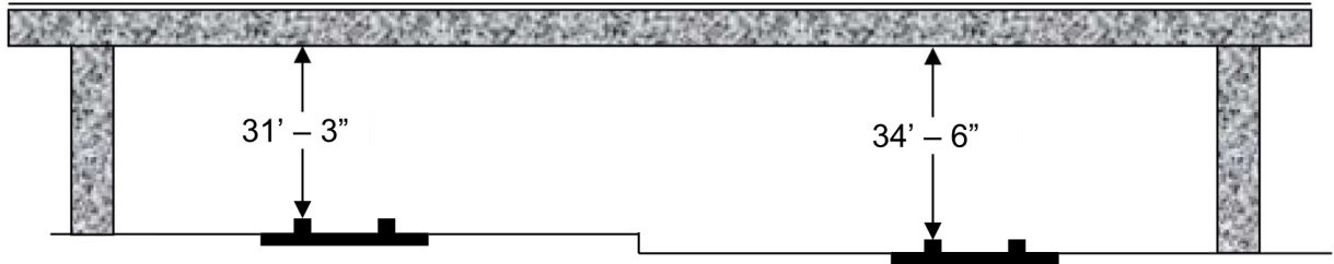
Railroad 31'- 3" beneath structure
