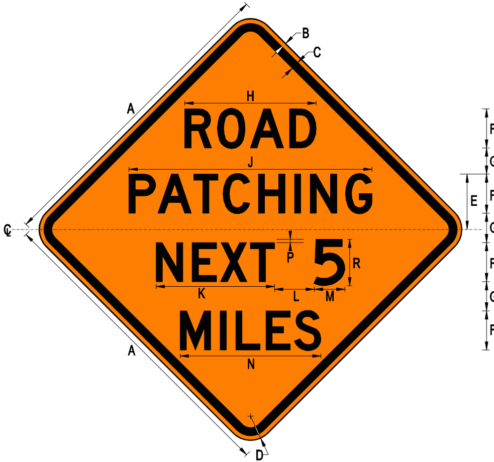
W21-V19 ROAD PATCHING NEXT 5 MILES
