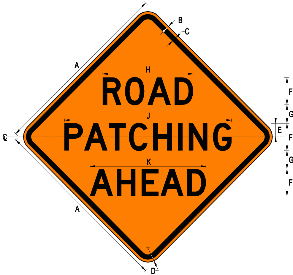
W21-V18 ROAD PATCHING AHEAD
