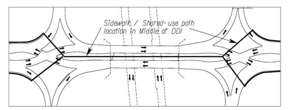
FIGURE \*A3-18 PEDESTRIAN ACCESS IN MIDDLE OF CROSSROAD BETWEEN CROSSOVER
