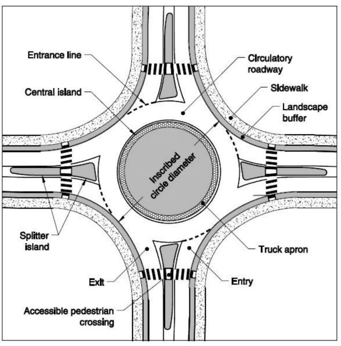
FIGURE A3-7 ROUNDABOUT DESIGN ELEMENTS\*
