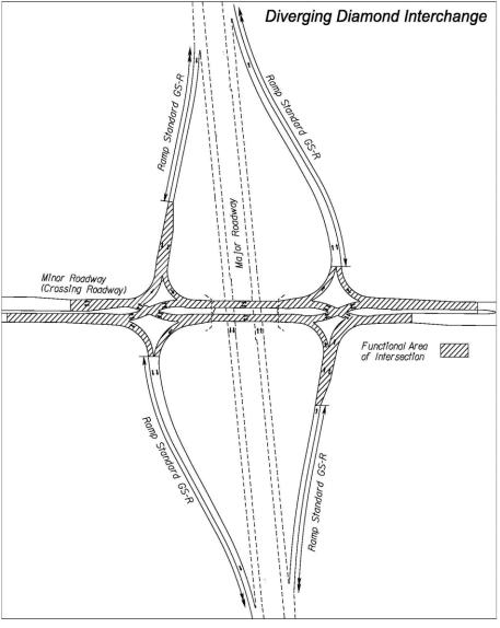
FIGURE A3-13 FUNCTIONAL AREA OF A DDI INTERSECTION\*
