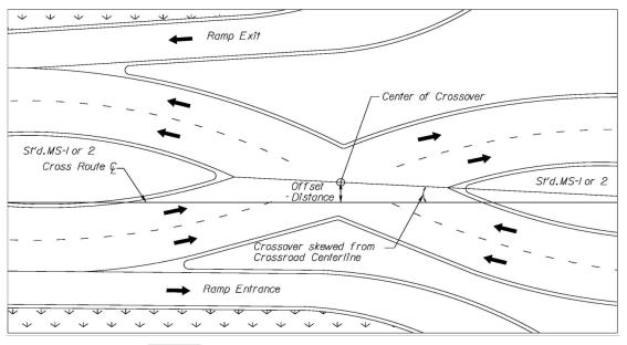
FIGURE A3-15<sup>\*</sup> OFFSET DISTANCE FOR INTERSECTION
