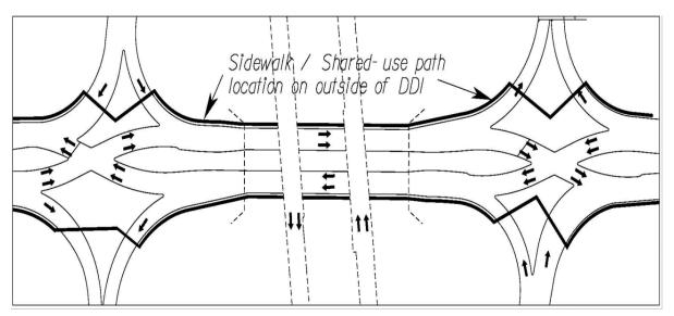
FIGURE A3-19 PEDESTRIAN ACCESS OUTSIDE OF DDI
